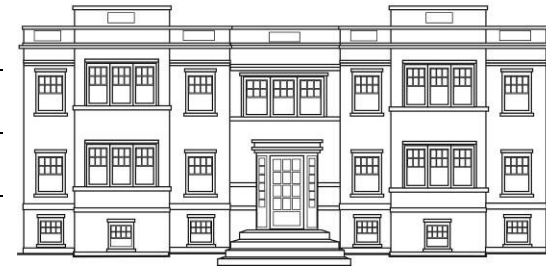
Pedestrian entrance facing sidewalk Parking to side or rear First floor elevation minimum 3 feet above sidewalk
